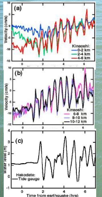
Time series of velocity components from the Kinaoshi radar (42 MHz transmitter frequency) and simultaneous water level observations from the Hakodate tide **Radial velocity was** resolved gauge. perpendicular to the shore, and averaged over bands 2 km wide parallel to the depth contours.
