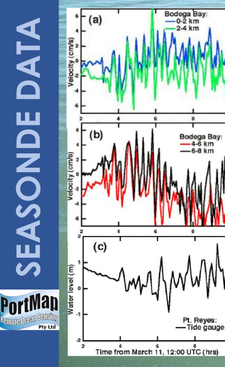
Time series of velocity components from the radar Bodega at Bay and simultaneous water level observations from the Point Reyes tide gauge in California, USA. Radial velocities were resolved perpendicular to the shore, and averaged over bands 2-km wide parallel to the shore. The radar has 13 MHz transmit frequency and 2 km range increments.
