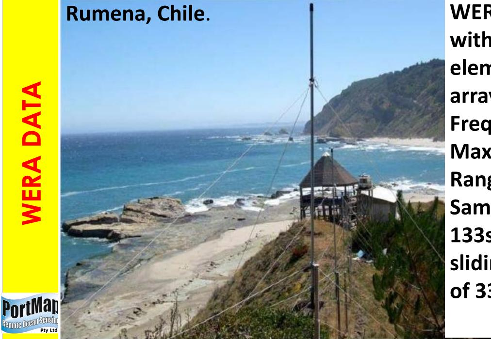
**WERA Radar** with an 8element phased array. Freq 22 MHz Max range 50km Range res:0.6km Sampling on 133s time series sliding in steps of 33s.
