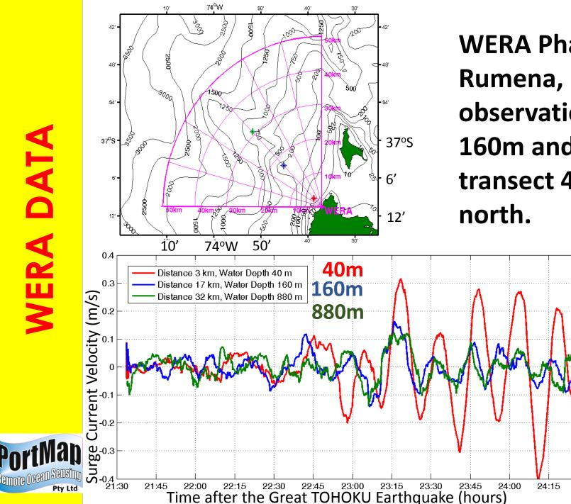
WERA Phased Array radar at Rumena, Chile made observations at depths 40m, 160m and 880m along the transect 45 degrees west of north.
